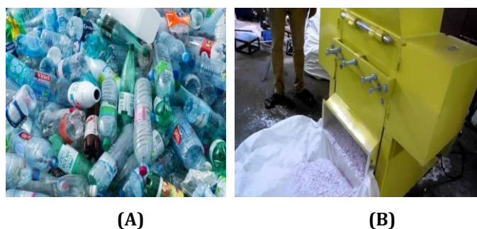
Fig-1 (A) Polyethylene waste before cutting and grinding after cutting (B) Grinding polyethylene Waste
