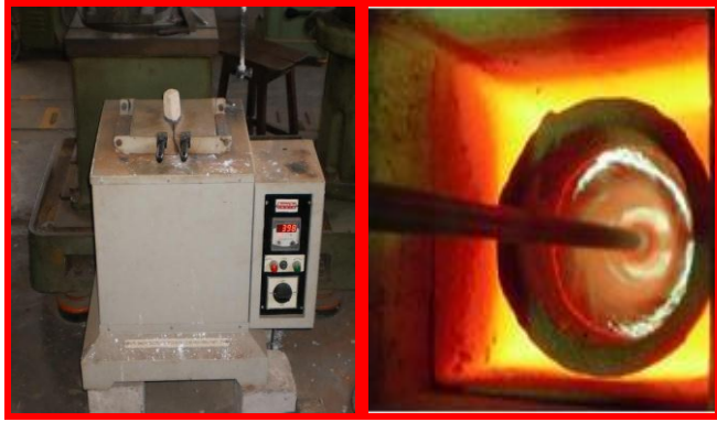
Fig-3: Muffle Furnace and Samples in Muffle furnace
