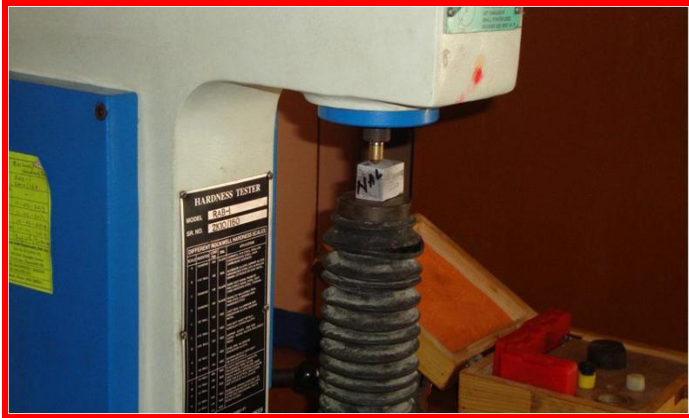
Fig-6: Brinell hardness test equipment setup.
