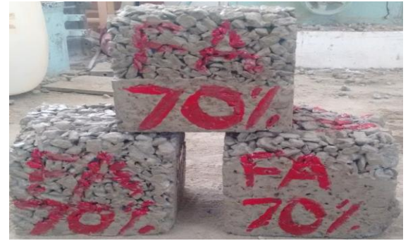
FIGURE 14 PERVIOUS CONCRETE CUBES WITH 70%FA+30%CEMENT
