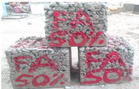
FIGURE 13 PERVIOUS CONCRETE CUBES WITH 50%FA+50%CEMENT
