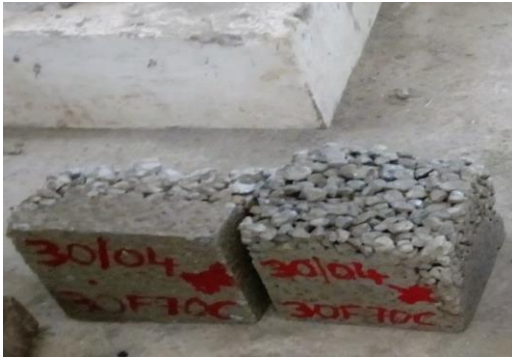
FIGURE 12 PERVIOUS CONCRETE CUBES WITH 30%FA+70%CEMENT
