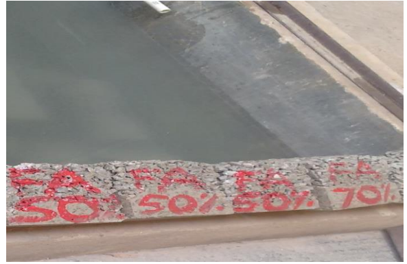
FIGURE 10 PLACING CUBES FOR CURING
