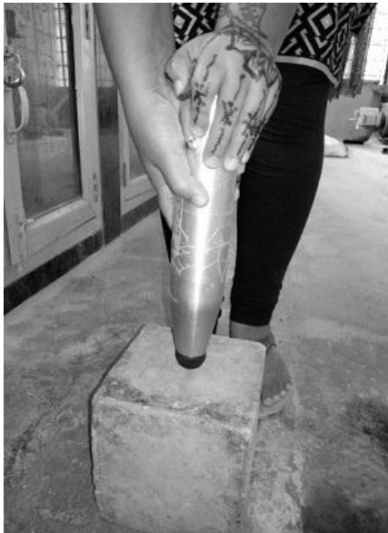
Figure 4: Test Setup for Rebound Hammer
