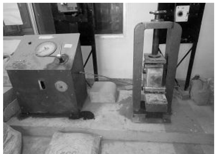
Figure 3: Test Setup for Flexural Strength
