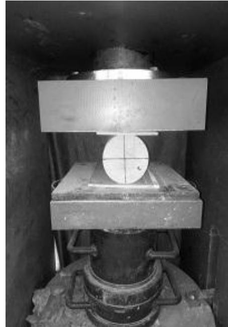
Figure 2: Test Setup for Split Tensile Strength
