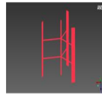
Fig. 3.7 H-Rotor model at H/D=1.8
