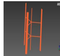
Fig. 3.9 H-Rotor model at H/D=2.2
