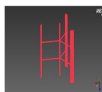
Fig. 3.5 H-Rotor model at H/D=1.54
