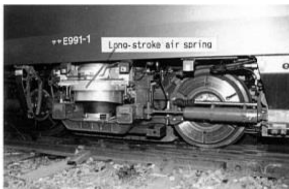
Fig 4 (a) Long-Stoke Air Spring Mounted on Bogie
