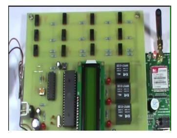
Fig.04: Testing Microcontroller & GSM Modem.
