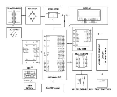
**Fig.03:** Block Dig. Of Design & Implementation of Fault Identification In Underground Cable Using IOT.
