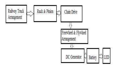
Fig.-1 Block Diagram of Generation of Power Using Railway Track
