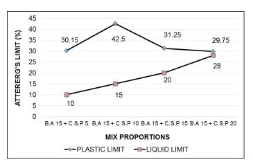
**Chart -6**: 15% Bottom ash with varying the Coconut Shell Powder by 5%, 10%, 15%, 20%
