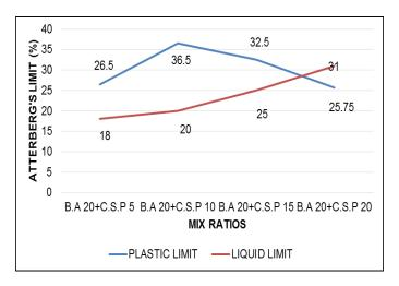
**Chart -7**: 20% Bottom ash with varying the Coconut Shell Powder by 5%, 10%, 15%, 20%
