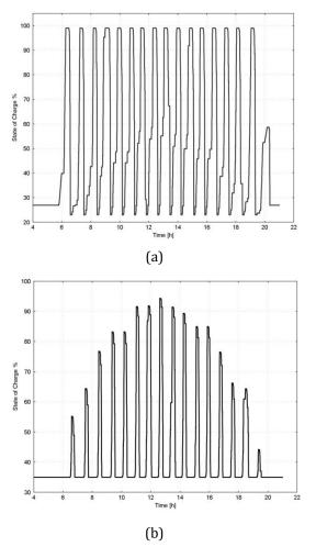
Fig. 4: Variation of the SOC of (a) primary battery (b) backup battery
