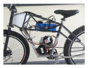
Fig-4: The ride monitoring module mounted to an E-Bike
