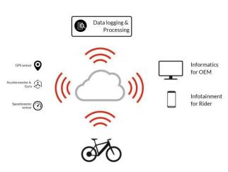
Fig-1: Connected E-Bike system
