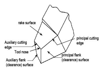
Fig-1: Features of a single point tool
