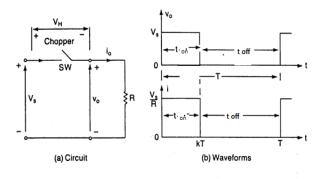
Fig-1: DC Chopper Circuit And Waveforms
