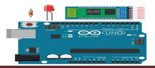
Diagram 2.4.1: arduino with Bluetooth device[1]
