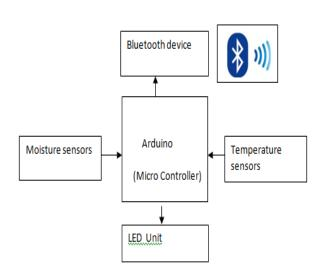
Figure 1: block diagram of monitoring unit
