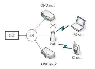
Figure 1: RoF Wi-Fi access network architecture: PON and its wireless extension RAU
