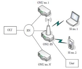
Figure 2: R&F Wi-Fi access network architecture: PON and its wireless extension ONU-BS
