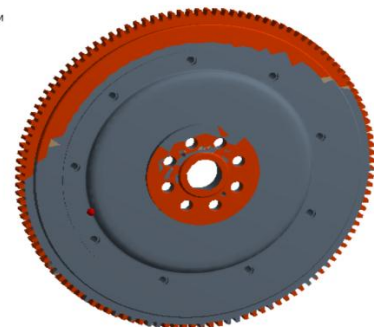
Fig. 16- Optimization result for Al Alloy Flywheel.
