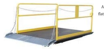
surface that is raised higher than the floor or ground and that people stand on when performing. In hydraulic ladder it gets up and we can perform our work. It having a rod surrounding to platform for the safety precaution of person or workers. Top platform is made of mild steel angle having dimension 1.8 × 3.1 feet and height of platform is 2.3 feet.
