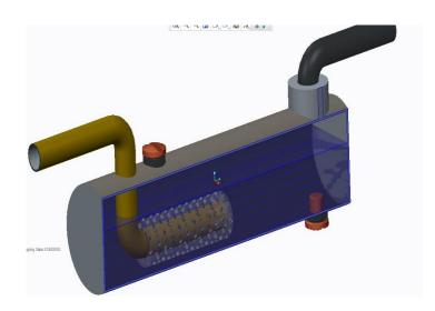
Fig – 5: Sectional view of aqua silencer
