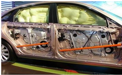
Fig -4: Hyundai Azera showing the side impact beams and the side impact airbags deployed.
