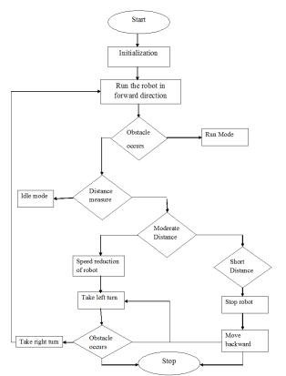
Fig.3: Obstacle Avoidance Flowchart
