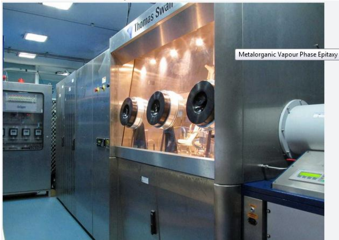
Fig -1: Metal organic vapour phase epitaxy
