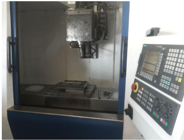
Fig. 2 Experimental setup describing FSW using VMC machine
