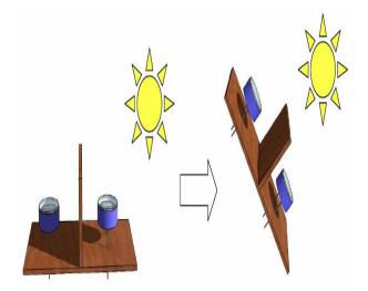
Figure 1. Sensor response once a shadow is cast on one LDR
