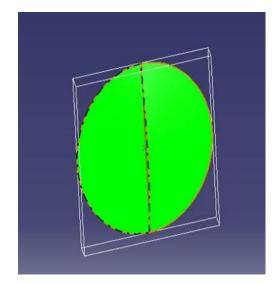
Figure 3.Scheffler-Type Solar Concentrator (STSC)
