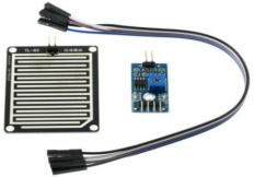
Fig -6: Rain Sensor Module (YL-83)
