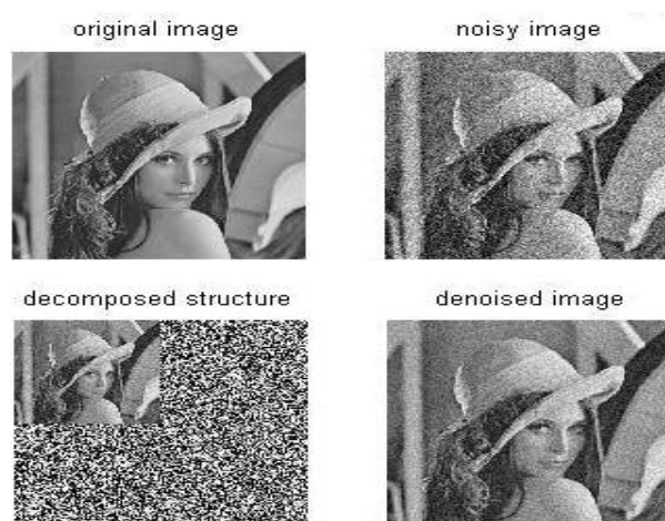
Figure 8: Result of AWGN noisy lina using haar second level Decomposition with Soft thresholding.
