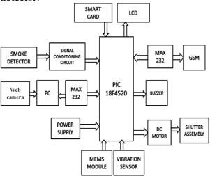
Fig.1 Block diagram of ATM Machine Security System Using GSM and MEMS sensor.
