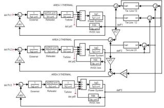
Figure 1. Three Area interconnected Power system with HVDC link
