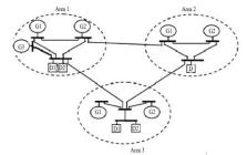
Figure2: Block Diagram of Three area Open Market System
