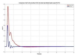
Fig 6: With and Without HVDC Link Area2 delta F using <u>PSO-PID</u> under open market system.
