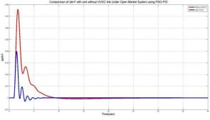
Fig 7: With and Without HVDC Link Area3 delta F using <u>PSO-PID</u> under open market system.
