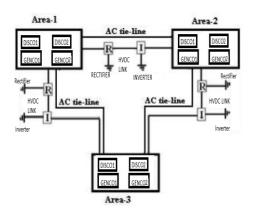
Figure 3: Configuration of Three-Area Power system With HVDC link.
