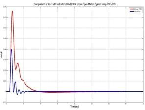
Fig 5: With and Without HVDC Link Area1 delta-F using <u>PSO-PID</u> under open market system.
