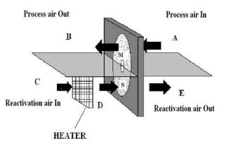
Fig -2: Working of solid desiccant Air conditioning<sup>[2]</sup>
