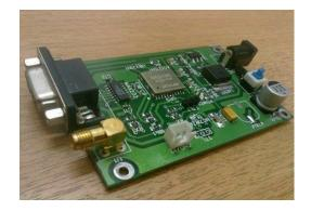
With a tiny configuration of 24mm x 24mm x 3 mm, SIM900 can fit almost all the space requirements in your M2M application, especially for slim and compact demand of design.
