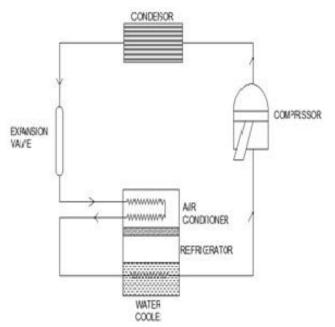
Fig-2: Project Circuit Diagram
