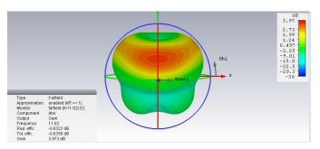
Fig -8: Gain of the proposed antenna
