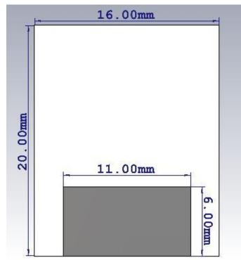
Fig -3: Back view of the proposed antenna
