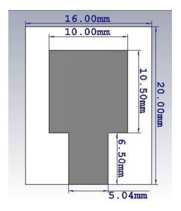
Fig -2: Front view of the proposed antenna
