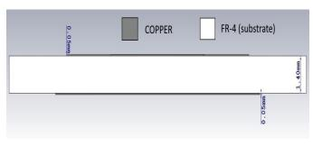
Fig -1: Side view of the proposed antenna
