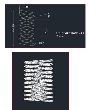
Fig – 7: Spring design for cad
