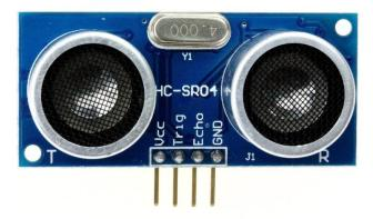
Fig. 2. Ultrasonic sensor
