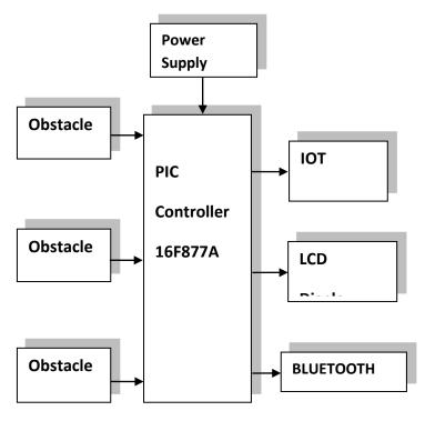
Fig -1: Block diagram of parking system
