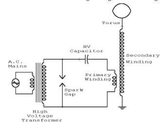
the capacitor. The capacitor is connect in series with the primary coil of output transformer. When the voltage value reaches to high enough to breakdown the spark gap, a spark will bridge the spark gap and complete the circuit between the capacitor and primary coil by shorting the transformer.
