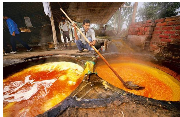
Fig1: Heating and separation of impurities
