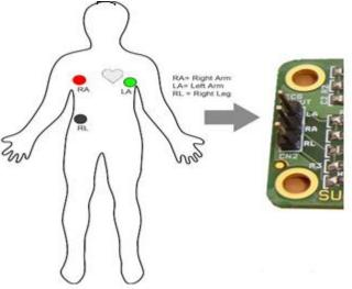
Fig-5: Connection for the ECG Sensor
