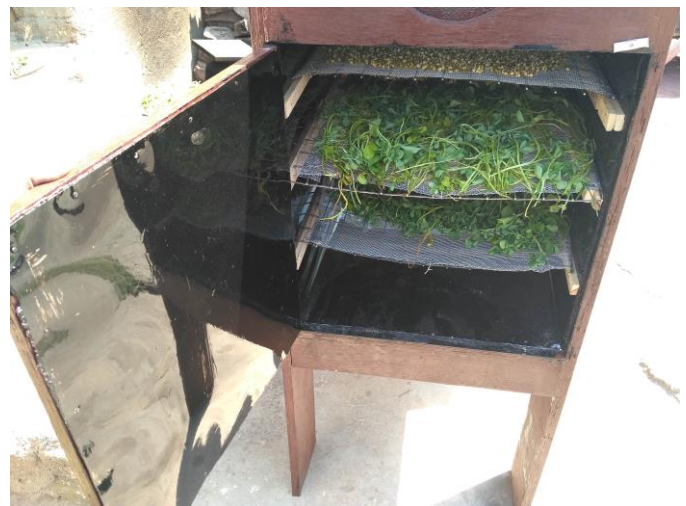
1.4 Drying Chamber with Trays
