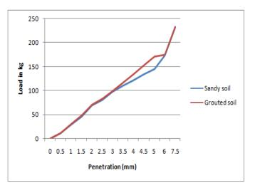
Graph.3. California bearing ratio test value
