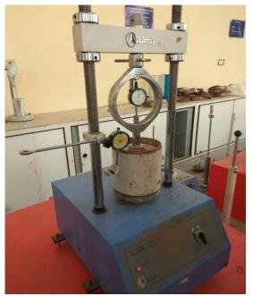
Fig.4. California bearing ratio test
