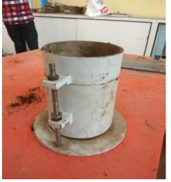
Fig.3. Proctor compaction mould
