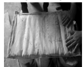
Fig-4: Modified Concrete cloth
