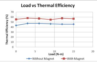
Chart -3: Load vs. Thermal efficiency
