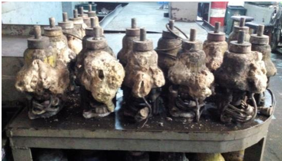
Figure No. 3: Glauber's salt on pot motor
