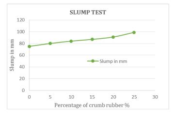
Fig -1: Variation in slump of rubber incorporated concrete specimens
