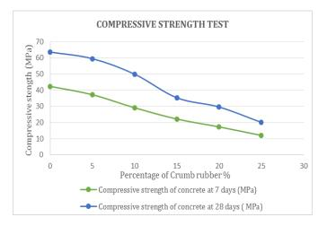
Fig -2: Variation in compressive strength of rubber incorporated concrete specimens
