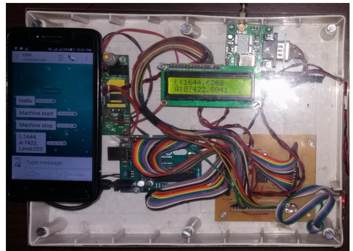
Fig-5: Hardware of Excavator monitoring and auto reporting using GSM.
