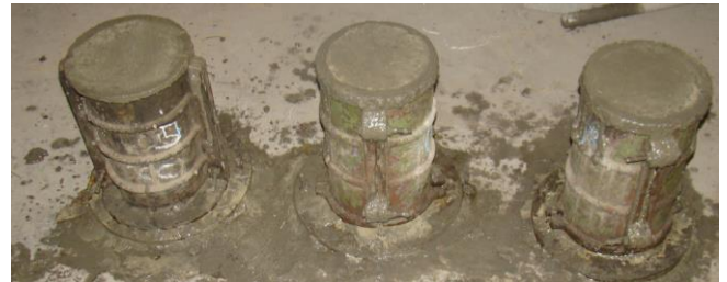
Fig 4: Cube and Cylinder specimens
