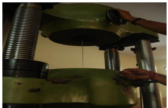
Fig 2: Tension test on steel wire
