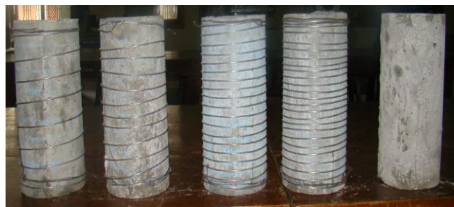
Fig 7: Confined Cylinder specimens
