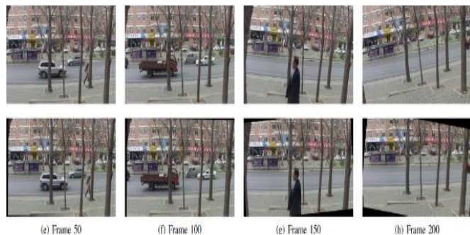
Fig. -5: Experimental result [4]. First row shows un-stabilized video sequence. Second row shows stabilized video sequence.
