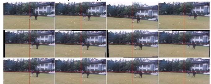
Fig. -2: Result of video stabilization [2]. First row: original input sequence: frame numbers are 5, 10, 15, 20. Second row is stabilized sequence with missing areas. Third row stabilized and mosaicing sequence
