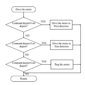
Microcontroller is used to drive the motor to the clockwise direction when the command degree is greater than the last degree and counterclockwise direction when the command degree is less than the last degrees in Figure.. And it is used to drive the motor
