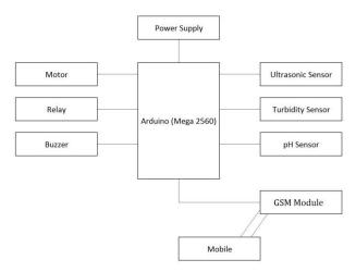
Fig-1 Block diagram of the Chlorine level controller
