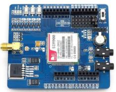
Fig -6: GSM Sim 900
