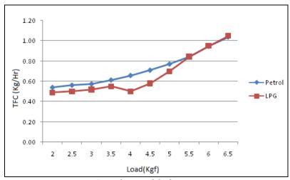
Figure: 3 Load vs total fuel consumption
