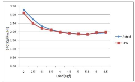
Figure: 4 Load and specific fuel consumption
