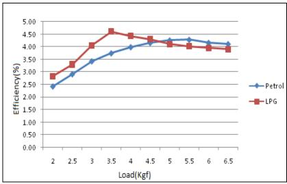
Figure: 5 Load vs brake thermal efficiency
