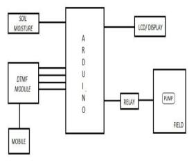
Fig -1: Block diagram of module
