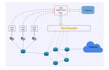
Fig -1: The QoS/QoE adjustment model architecture
